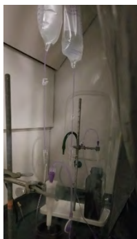
Set up used to concentrate thiamine from water samples
